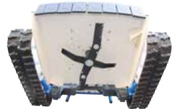
**Mower Deck** strong and versatile which allows to process high volume of grass and brush in both drive directions to avoid danger manouvre on the slope.
