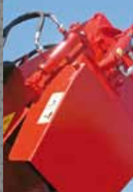
Hydraulic command for the deflector.
