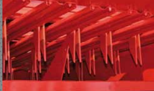
The loading conveyor can be equipped with 5 knives (in the picture only 1).
