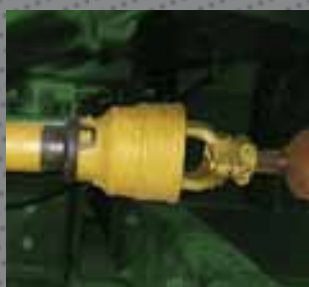
Transmission to the augers by cardan shaft with security bolt.
