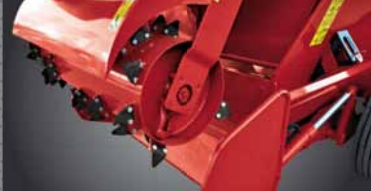
Cutter with 8 knives on the side for better loading.
