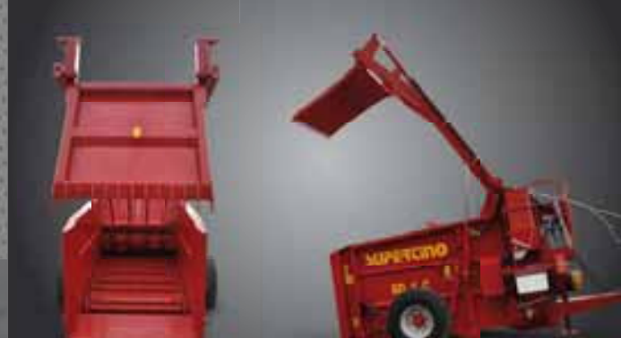
Silo arm for loading bales and silo products. (Self loading).
