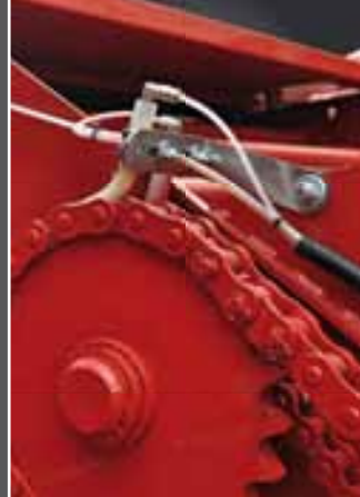
Automatic lubrication of chains.
