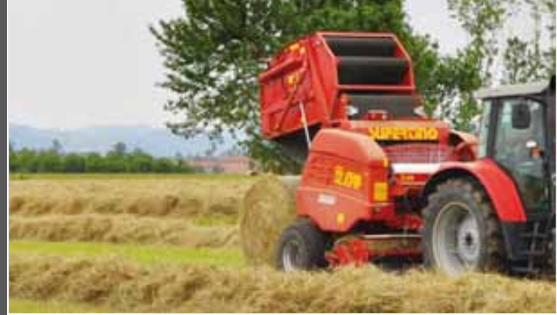
Adjustable diameter of the bale from 90 till 170 cm.
